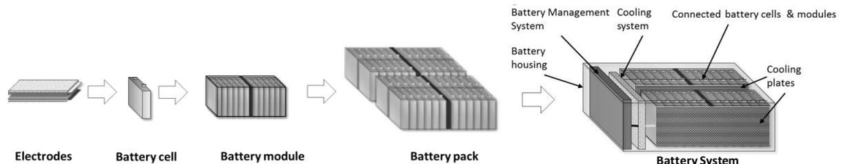
Figure 1: Schematic overview of the key components of a battery system after (Hettesheimer 2017)
